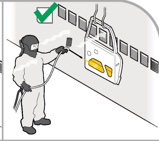
FIGURE 4 Spraying with a 'long' nozzle avoids overspray of the operator
