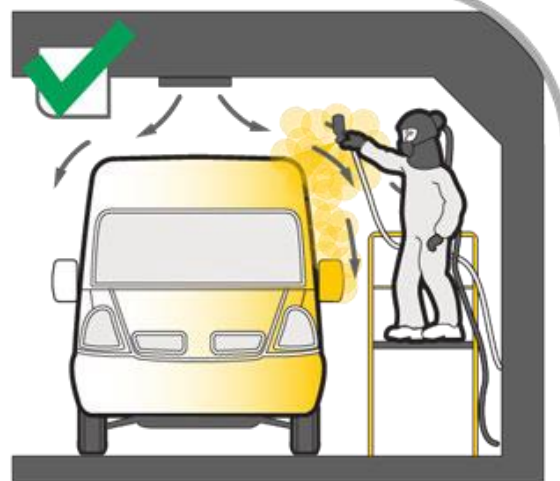
FIGURE 8 The use of a gantry or lift avoids overspray on to the operator, and avoids them having to stretch and reach
