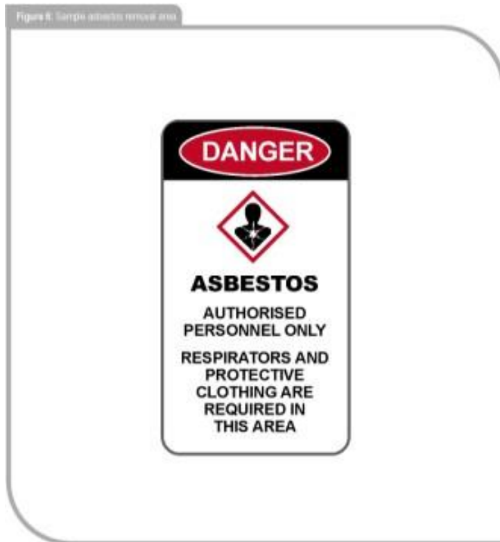
Figure 1 An example asbestos removal area sign
