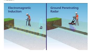
Electromagnetic Induction uses a transmitter to energise the utility with a current, setting up an electromagnetic field. This is then detected using a receiver.
