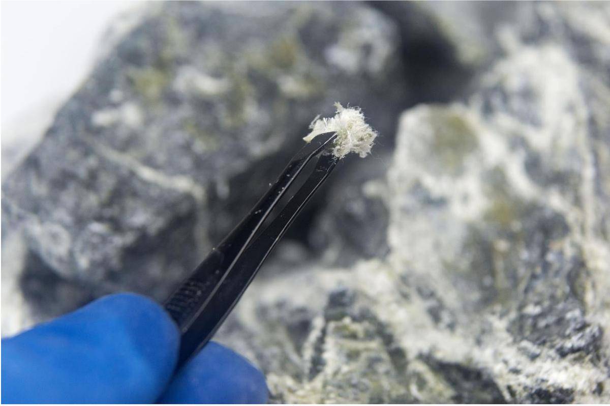
Chrysotile asbestos (white) is the most common type of asbestos used in Australia.
