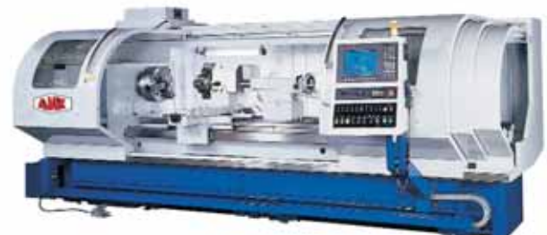
CNC (Computer Numeric Control) lathe: Substituting a centre lathe with a CNC lathe is an example of improved risk control of machinery and equipment through improvement in design.
