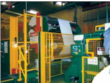
Fences, barriers, guards and interlocked gates separate people from the hazardous action of machinery and equipment.
