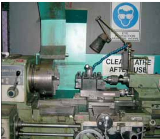
Centre lathe: The exposed rotating chuck of a centre lathe can eject parts or tools with great force, cutting fluid fumes are difficult to contain and the machinery requires manual set-up.
