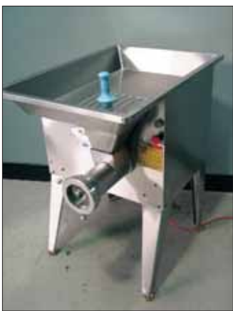
The covered throat of the mincer prevents a person's hand from accessing the hazard.
