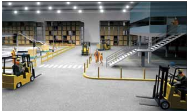
Mobile plant operated in areas where people work may cause injury through collision. Traffic control and segregation are forms of control.
